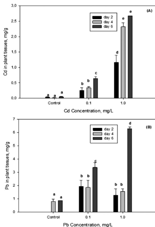
**Figure 5.** The accumulation of Cd (A) and Pb (B) by *Lemna gibba* at different concentrations and exposure times. Values represent mean  $\pm$  S.D. Different letters indicate significant differences ( $P < 0.05$ ) according to the ANOVA test.
